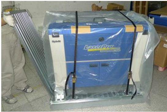
Step 4: Fix the four side boards by four corner brackets.
